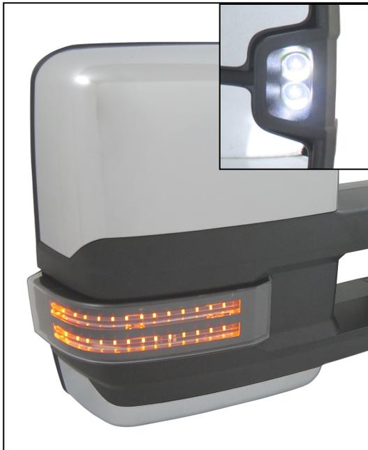
1. This multi-signal installation overview will show you what extra light features are provided on our mirrors. If the plug on your vehicle doesn't have pre-wired pins to power the **1. Turn Signal 2. Marker Lamp 3. High-Power LED Spotlight**, then you will need to use the included hardware to hardwire these lights into their appropriate circuits.
